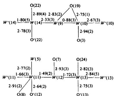
Fig. 4. Distances (Å) in the environments of the clusters of lattice water molecules. Those four water molecules which are equivalent by centers of inversion are denoted by  $W'$ .
